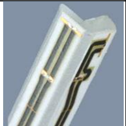
Fig 5.2 Photo of E-field Probe
