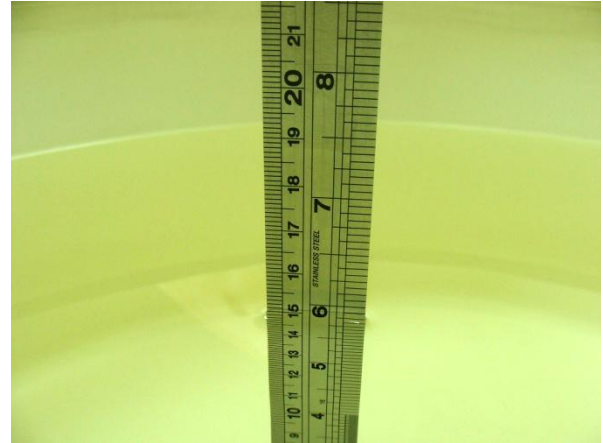
Fig 6.2 Photo of Liquid Height for Body SAR
