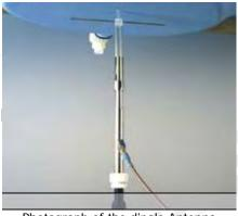
Photograph of the dipole Antenna
