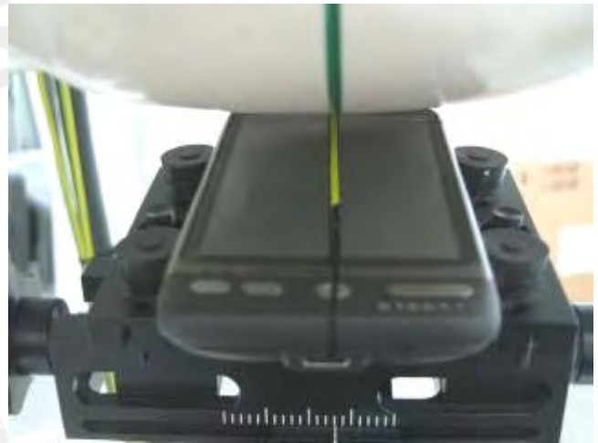
Fig.6 Left Head Section / Ear-Tilt Position(15°)
