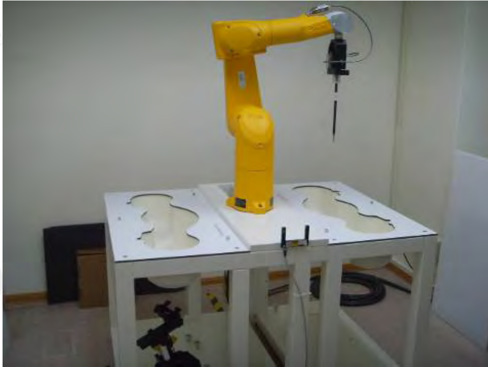
Fig.1 Photograph of the SAR measurement System
