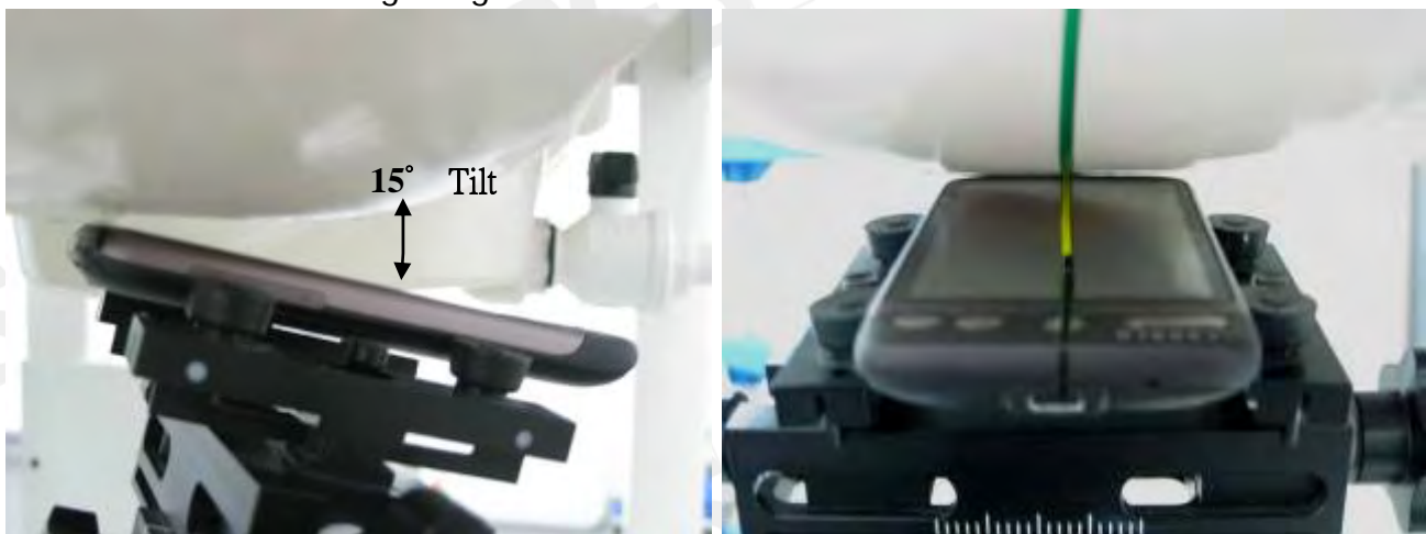
Fig.4 Right Head Section / Ear-Tilt Position(15°)
