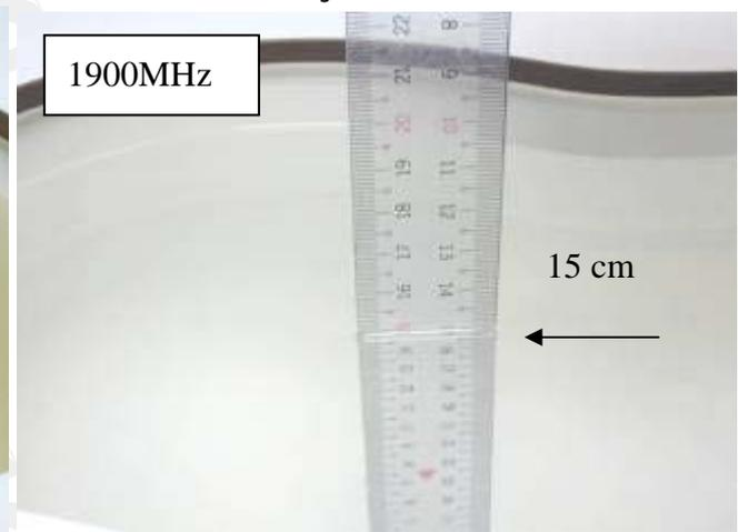
Fig.2.2 Photograph of the Tissue Simulant Fluid liquid depth 15cm for Right-head Side
