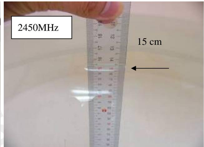
Fig.2.6 Photograph of the Tissue Simulant Fluid liquid depth 15cm for Flat (Body)
