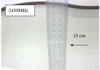
Fig.2.5 Photograph of the Tissue Simulant Fluid liquid depth 15cm for Right-head Side Fig.2.4 Photograph of the Tissue Simulant Fluid liquid depth 15cm for Flat (Body)
