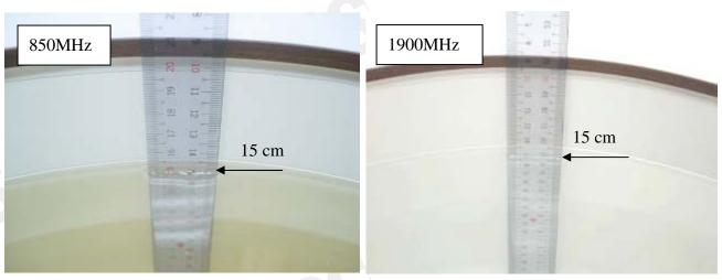
Fig.2.3 Photograph of the Tissue Simulant Fluid liquid depth 15cm for Flat (Body)
