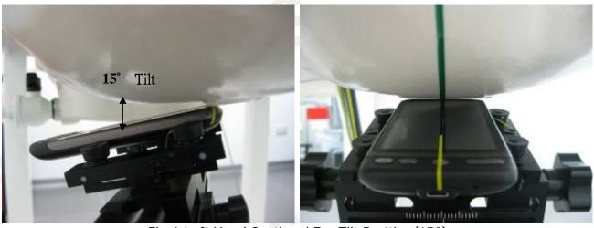
Fig.6 Left Head Section / Ear-Tilt Position(15°)
