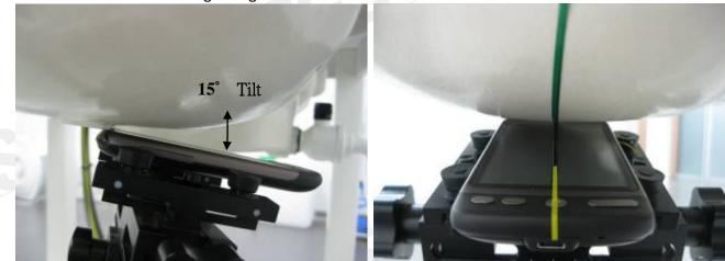
Fig.4 Right Head Section / Ear-Tilt Position(15°)
