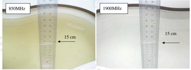
Fig.2.1 Photograph of the Tissue Simulant Fluid liquid depth 15cm for Left-head Side
