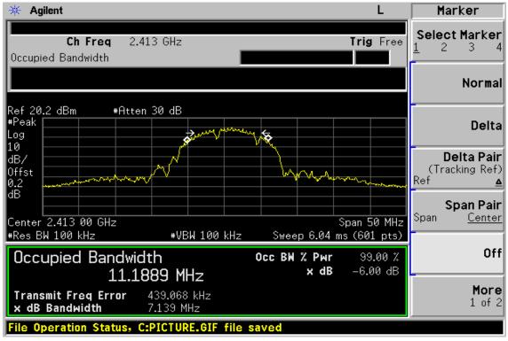
6dB Band Width & 99% Bandwidth Test Data CH-Mid
