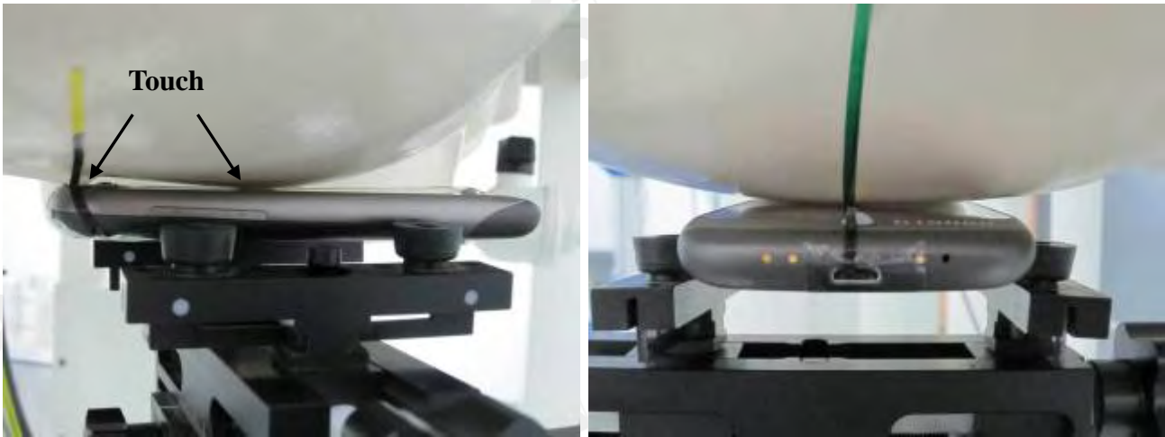
Fig.3 Right Head Section / Cheek-Touch Position
