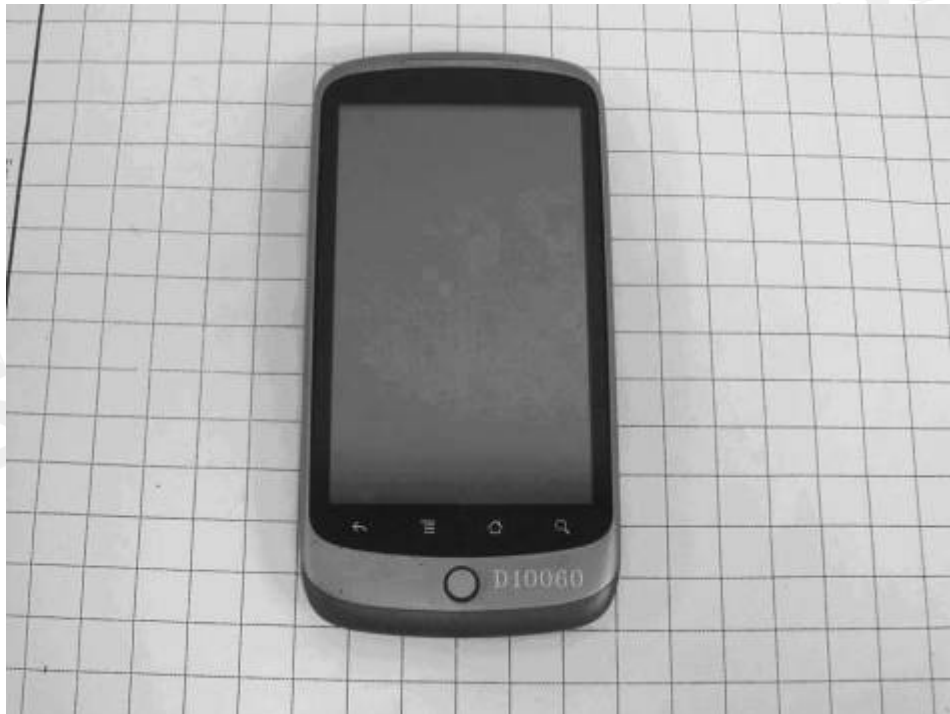
Fig.19 Second solution (change Camera) LCM Model No: AMS369FG03-0 Supplier: SAMSUNG Camera Model No:08PM15B Supplier: LITEON
