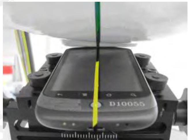
Fig.6 Left Head Section / Ear-Tilt Position(15°)
