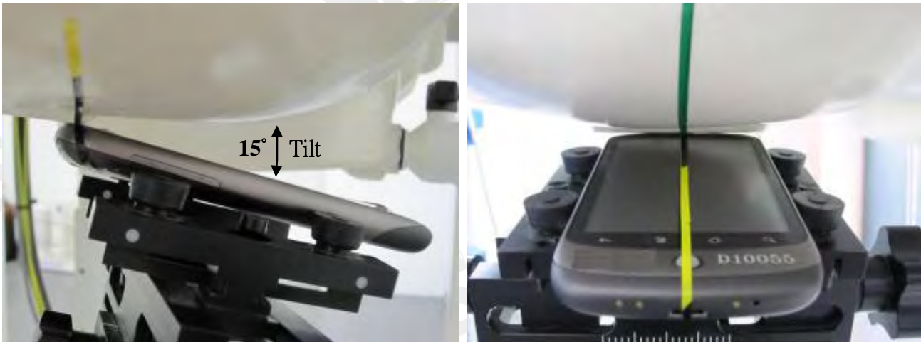
Fig.4 Right Head Section / Ear-Tilt Position(15°)
