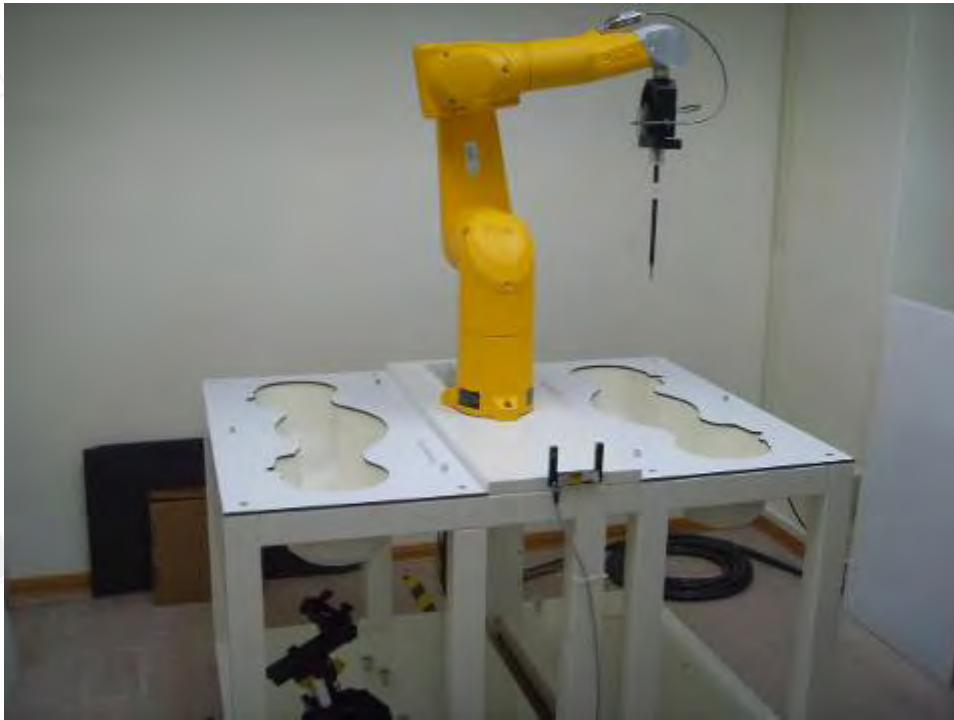
Fig.1 Photograph of the SAR measurement System
