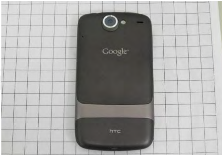
Fig.11 Back view of device LCM Model No: AMS369FG03-0 Supplier: SAMSUNG Camera Model No:08PM15A Supplier: LITEON
