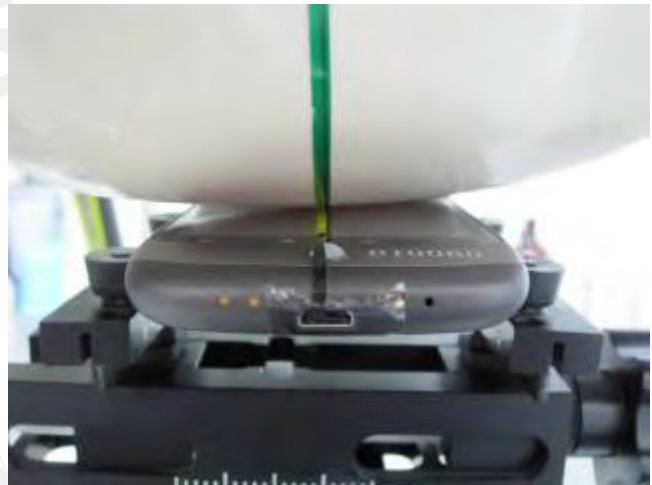
Fig.5 Left Head Section / Cheek-Touch Position
