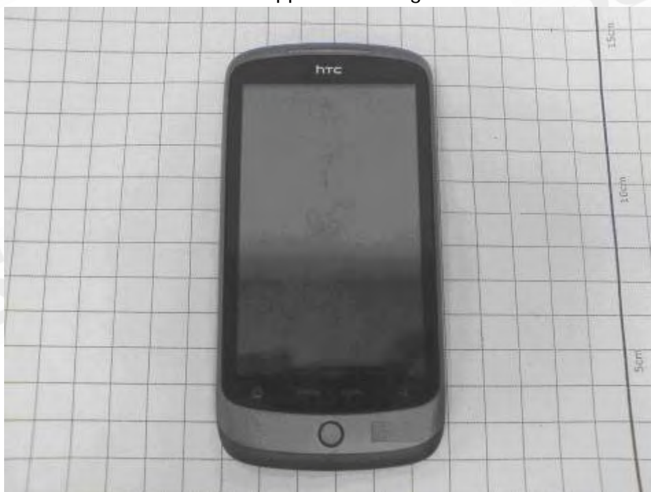
Fig.21 Second solution (change Housing painting & Camera) Camera Model No: 50-70483HTT8 Supplier: Primax
