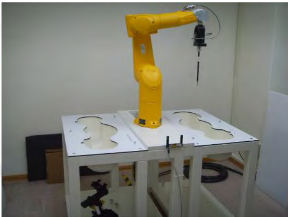
Fig.1 Photograph of the SAR measurement System
