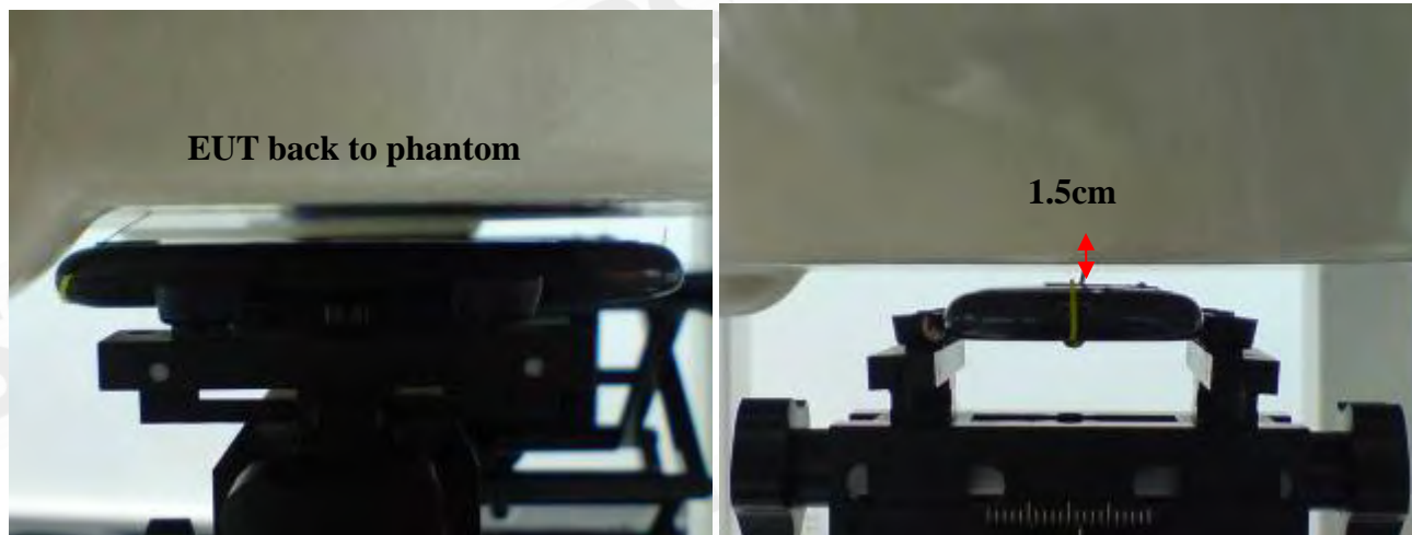
Fig.8 Body worn- EUT back to flat phantom and distance between flat phantom and mobile phone is 1.5 cm
