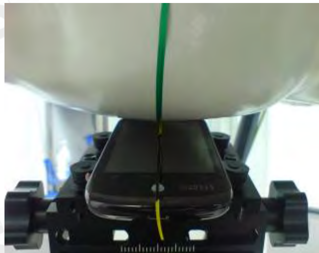
Fig.4 Right Head Section / Ear-Tilt Position(15°)
