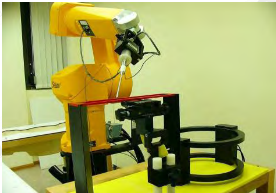
Fig.1 Photograph of the DASY 4 measurement System
