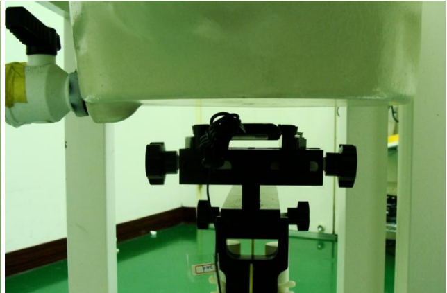
Bottom of the DUT with Phantom 1.5 cm Gap (DUT with Earphone 2)
