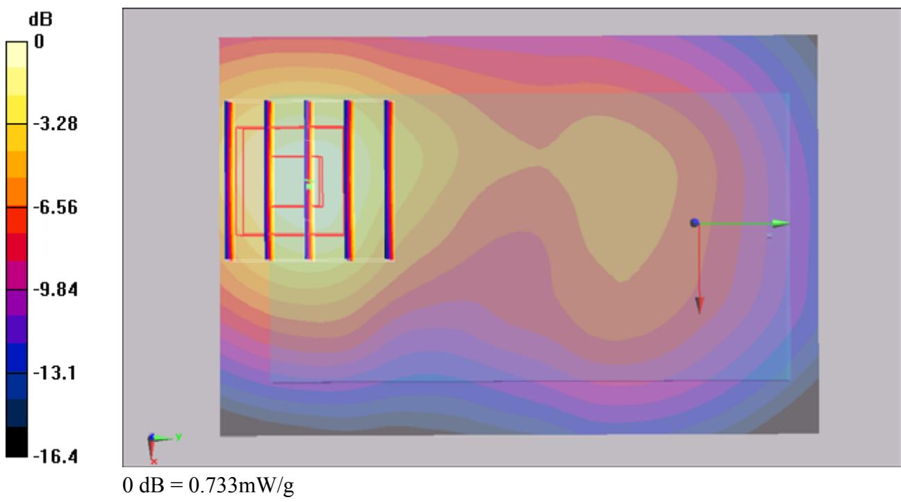
**#38 GSM1900\_GPRS10\_Bottom\_1.5cm\_Ch512\_Sample A\_2D****DUT: 011201**
