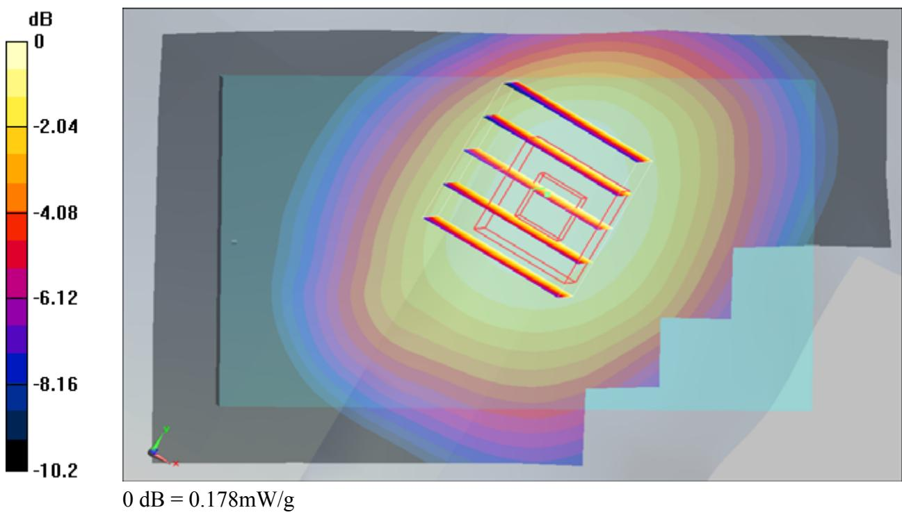
**#13 GSM850\_Right Cheek\_Ch251\_Sample1\_2D****DUT: 961306-03**
