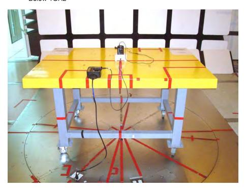
Description : Front View of Field Strength of Spurious Radiation Test
