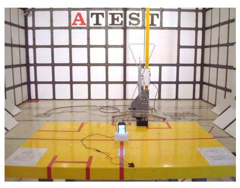
Description : Back View of Field Strength of Spurious Radiation Test
