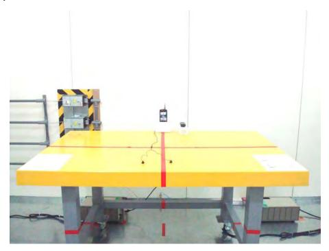
**Description**: Back View of Conducted Emission Test
