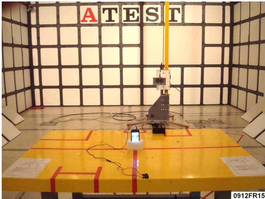
Description : Back View of Field Strength of Spurious Radiation Test Above 1GHz
