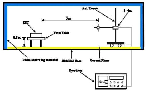
For the actual test configuration, please refer to the attached file (Test Setup Photo). **CONDUCTED POWER MEASUREMENT:**
