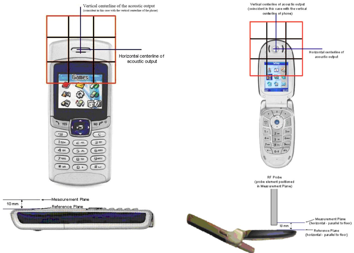
Fig 6.1 A typical DUT reference and plane for T-Coil measurements
