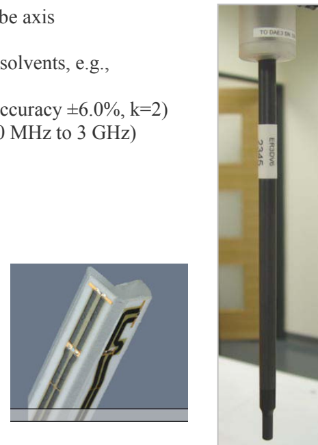
Figure 4 and 5: ER3DV6 E-Field Probe
