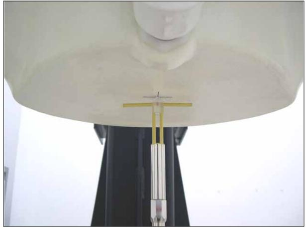
Fig 8.2 Dipole Setup
