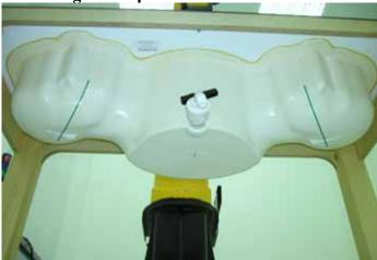
Fig. 5.4 Bottom View of Twin Phantom
