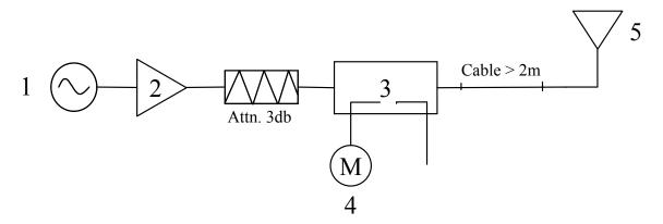
Fig. 8.1 System Setup for System Evaluation
