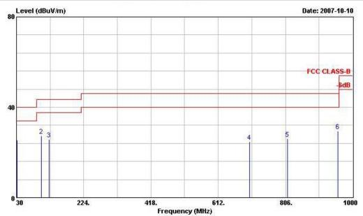
Site :03CH04-HY Condition:FCC CLASS-B 3m ANT2724 HORIZONTAL EUT :GSM/EDGE(Class12) 850/900/1800/ . :1900 UMITS/HSDPA 850/2100(BAND I and . :V) with BT\_EDR Phone\_Slide Type POWER :120Vac/60Hz MODEL :FR 792103 MOME :Bluetooth Tx\_Ch39;2441MHz DATA RATE:3DH1 PLANE :E2 ADAPTOR :B
