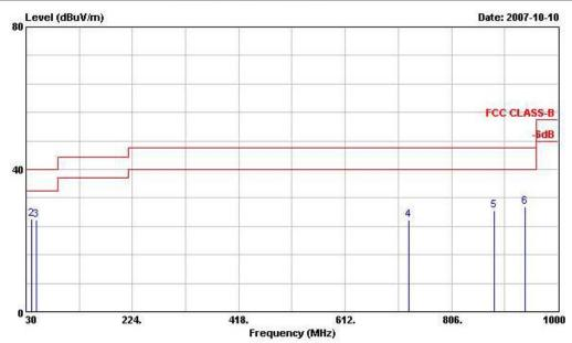
Site :03CH04-HY Condition: FCC CLASS-B 3m ANT2724 VERTICAL :GSM/EDGE(Class12) 850/900/1800/ EUT :1900 UMITS/HSDPA 850/2100(BAND I and . :V) with BT\_EDR Phone\_Slide Type :120Vac/60Hz POWER MODEL :FR 792103 :Bluetooth Tx\_Ch78;2480MHz MOME DATA RATE: 3DH1 PLANE : E2 ADAPTOR : B
