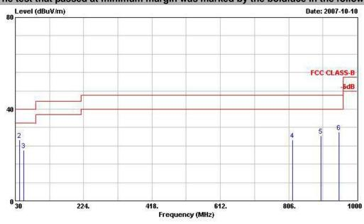
Site :03CH04-HY Condition: FCC CLASS-B 3m ANT2724 VERTICAL :GSM/EDGE(Class12) 850/900/1800/ EUT :1900 UMITS/HSDPA 850/2100(BAND I and  $\mathbf{x}_{i}$ :V) with BT\_EDR Phone\_Slide Type POWER :120Vac/60Hz MODEL :FR 792103 MOME :Bluetooth Tx\_Ch78;2480MHz DATA RATE:DH1 PLANE : E2 ADAPTOR : B PLANE
