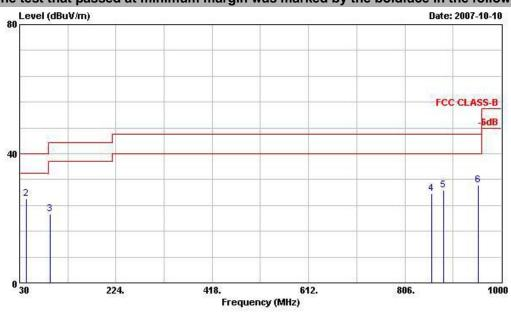
Site :03CH04-HY Condition: FCC CLASS-B 3m ANT2724 VERTICAL :GSM/EDGE(Class12) 850/900/1800/ EUT :1900 UMITS/HSDPA 850/2100(BAND I and  $\mathbf{e}_{i}$ :V) with BT\_EDR Phone\_Slide Type POWER :120Vac/60Hz MODEL :FR 792103 MOME Bluetooth Tx\_Ch78;2480MHz DATA RATE: 2DH1 PLANE : E2 ADAPTOR : B
