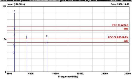
:03CH04-HY Site Condition: FCC CLASS-B 3m HF-ANT-6903 VERTICAL :GSM/EDGE(Class12) 850/900/1800/ EUT :1900 UMITS/HSDPA 850/2100(BAND I and 10 :V) with BT\_EDR Phone\_Slide Type POWER :120Vac/60Hz :FR 792103 MODEL MOME :Bluetooth Tx\_Ch78;2480MHz DATA RATE: 2DH1 PLANE : E2 ADAPTOR : B
