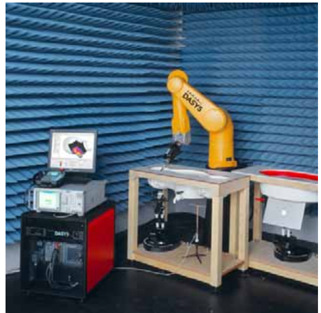
Fig. 5.2 Probe Setup on Robot
