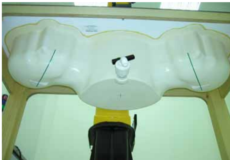
Fig. 5.4 Bottom View of Twin Phantom
