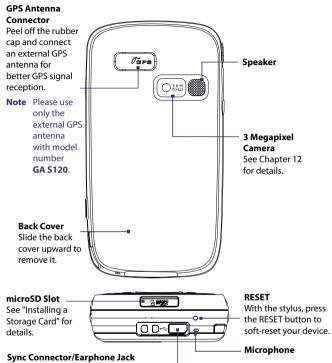
Connect the supplied USB cable to synchronize information or plug in the AC adapter to recharge the battery. You can also connect the supplied USB stereo headset for hands-free conversation or for listening to audio media.
