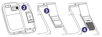
5. After inserting the USIM/SIM card, close the SIM card door and then lock it by sliding the lock to the right.
