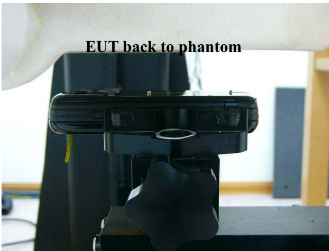
Fig.14 Body worn- EUT back to flat phantom and distance between flat phantom and mobile phone is 1.5 cm
