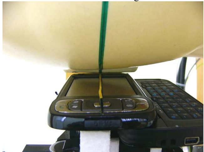
Fig.7 Right Head at Slider-on Section / Ear-Tilt Position(15°)
