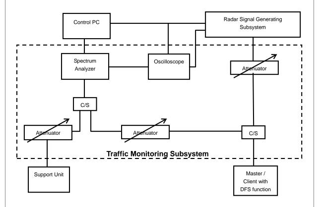
The test transmission will always be from the Master Device to the Client Device. While the Client device is set up to associate with the Master device and play the NTIA DFS MPEG file (6  $\frac{1}{2}$  Magic Hours) from Master device, the designated MPEG test file and instructions are located at: http://ntiacsd.ntia.doc.gov/dfs/.
