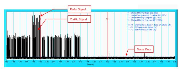
**NOTE:** An expanded plot for the device vacates the channel in the required 500ms.
