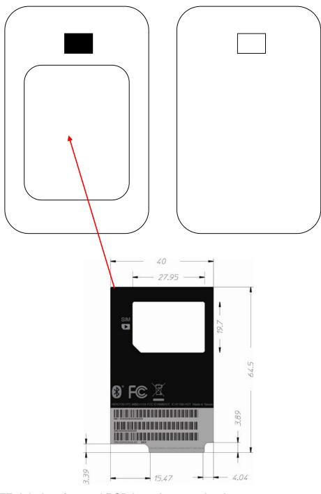
NOTE: label on internal PCB board, not on back cover
