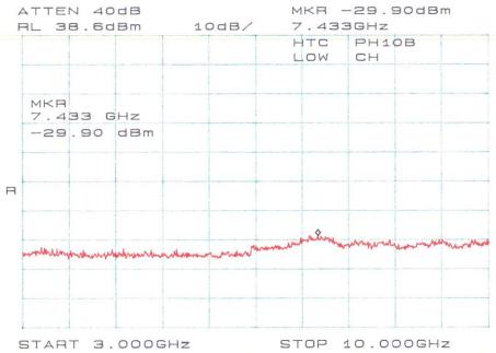
START 3.000GHZ STOP 10.000GHZ \*RBW 100KHZ VBW 100KHZ \*SWP 10.0sec
