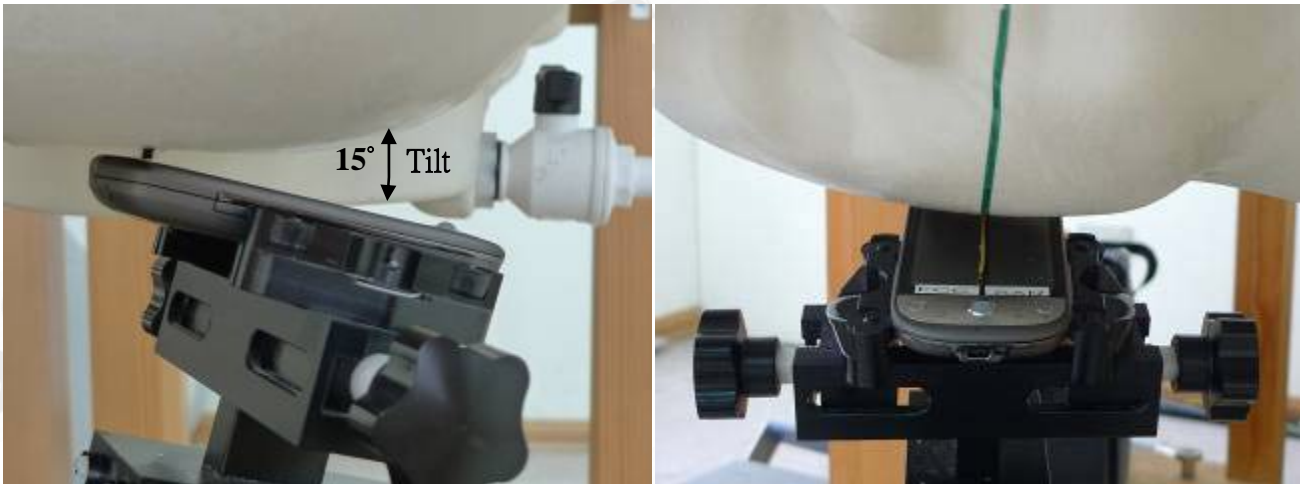
Fig.4 Right Head Section Ear-Tilt Position(15°)
