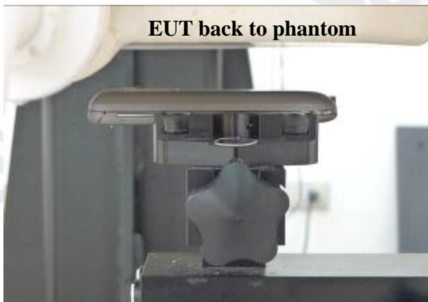
Fig.8 Body worn- EUT back to flat phantom and distance between flat phantom and mobile phone is 1.5 cm
