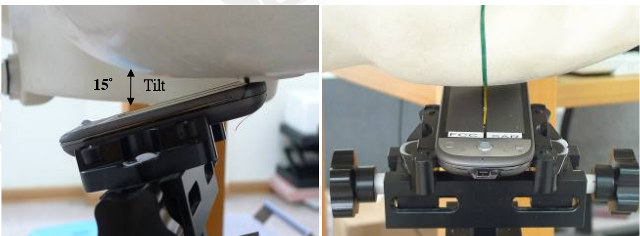
Fig.6 Left Head Section / Ear-Tilt Position(15°)
