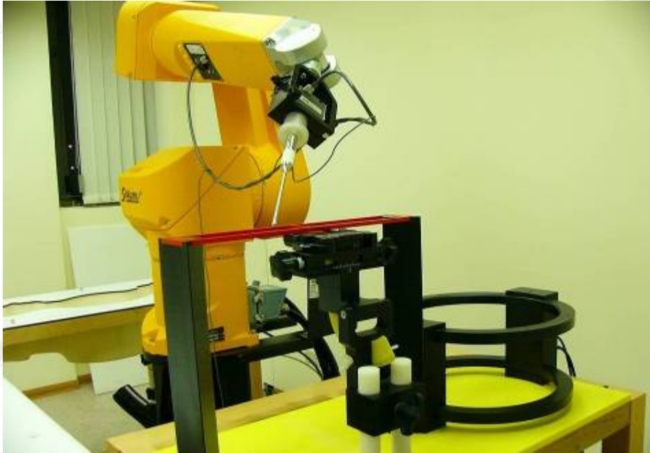
Fig.1 Photograph of the DASY 4 measurement System
