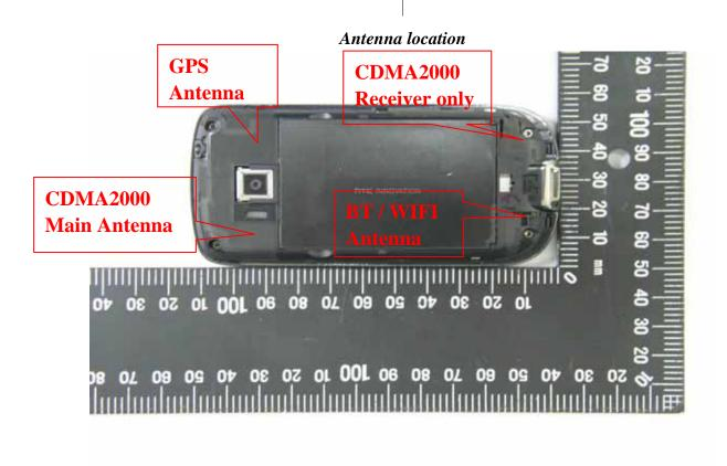
The min. distance is 6.3cm from CDMA2000 Antenna to WLAN/BT Antenna,
