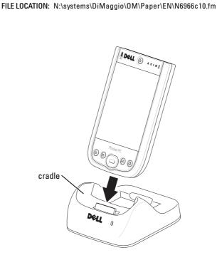
4 Align the connector on the bottom of the device with the connector on the cradle, and, keeping the front of the device flush with the front of the cradle, lower the device onto the cradle.
