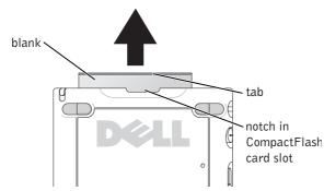
2 Align the tab on the back of the CompactFlash card with the notch in the CompactFlash card slot, and slide the card into the slot.
