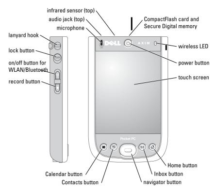
INFRARED SENSOR-The infrared sensor lets you transfer files from your device to
