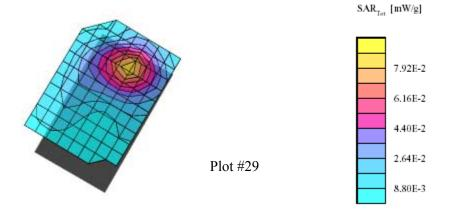
High Tech Computer, Model: PH20A2 (Left Head, Tilt, Mid Channel, Ambient Temp = 23 C, Liquid Temp = 22 C, 7/21/2004) SAM Phantom; Left Hand Section; Position: (90°,60°); Frequency: 1880 MHz
