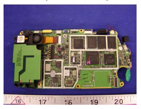
PH20A2 EUT – Solder View with Shielding
