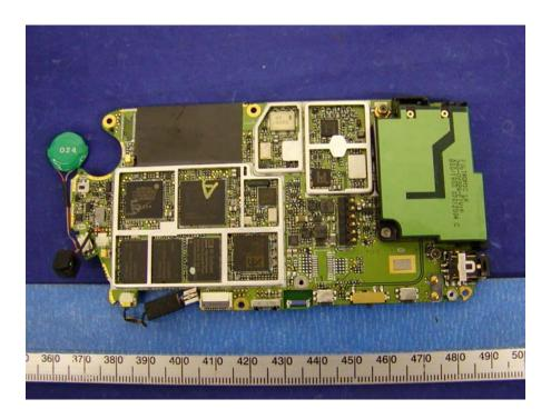
PH20A3 EUT – Solder View with Shielding
