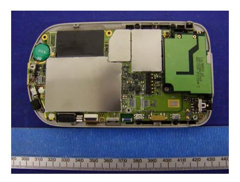
PH20A3 EUT - Component View with Shielding
