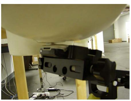
PH20A3, Body Worn, Back Touching Phantom with Headset, Memory Card and Pouch
