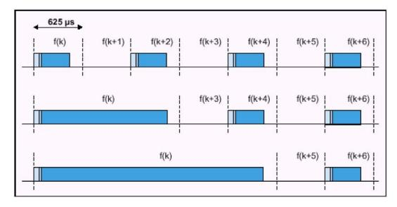
For DH5 packets the transmitter transmits across five 625 microsecond slots minus a guard band of 259 microseconds. The transmission is followed by a 625 microsecond receive slot. The transmission duty cycle (Tdc) for this case can be calculated as:
