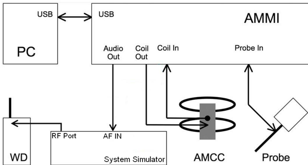
**Fig-3.2b T-Coil Setup Cabling for VoLTE**
