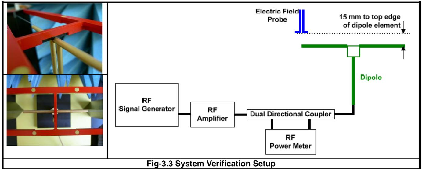
**Fig-3.3 System Verification Setup**
