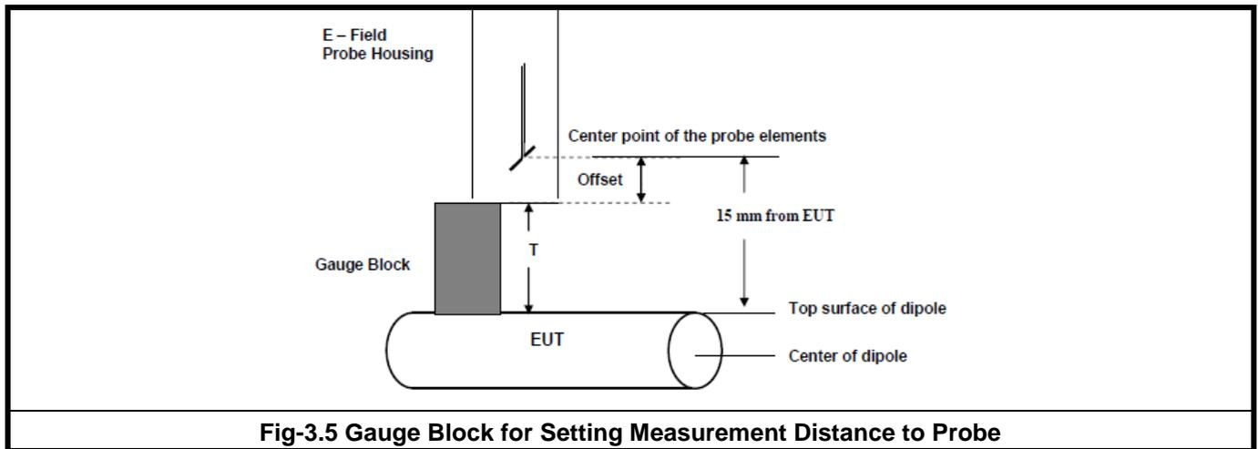
**Fig-3.5 Gauge Block for Setting Measurement Distance to Probe**
