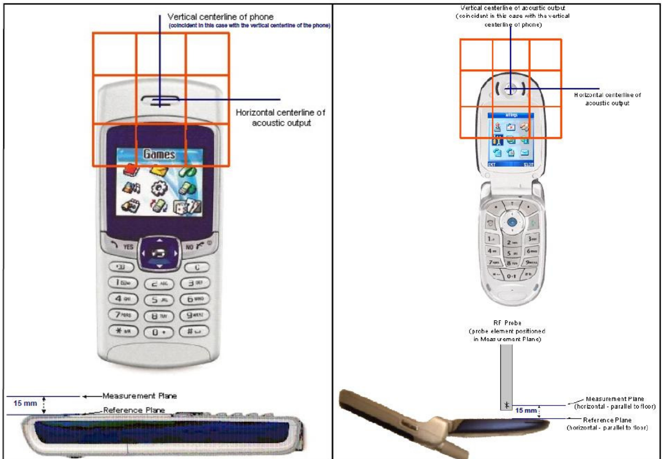
Fig-3.4 EUT Reference and Plane
