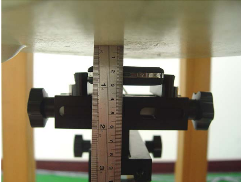
Fig. 9.7 Keypad Up with 1.5cm Gap
