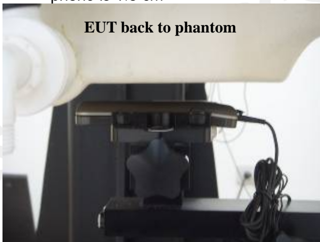
Fig.13 Body worn- EUT back to flat phantom and distance between flat phantom and mobile phone is 1.5 cm_repeated with handset
