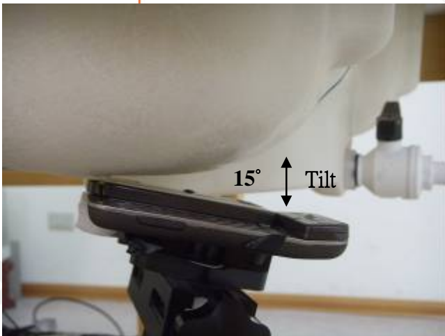
Fig.6 Right Head at Slider-on Section / Ear-Tilt Position(15°)
