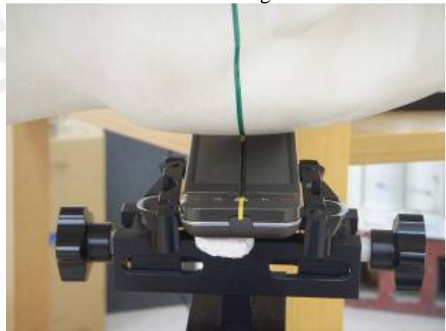
Fig.9 Left Head at Slider-off Section / Ear-Tilt Position(15°)
