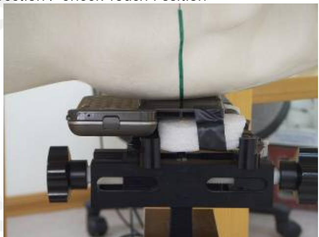
Fig.8 Left Head at Slider-on Section / Cheek-Touch Position
