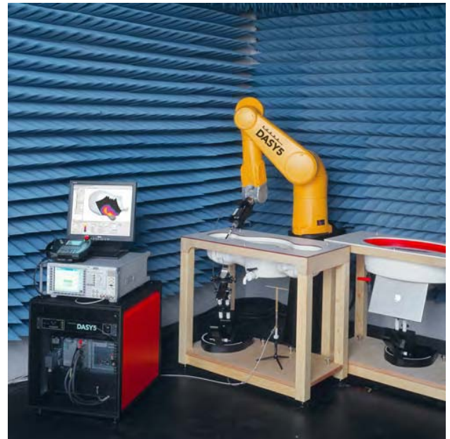
Fig. 5.2 Probe Setup on Robot
