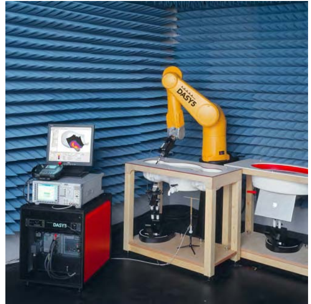
Fig. 5.2 Probe Setup on Robot
