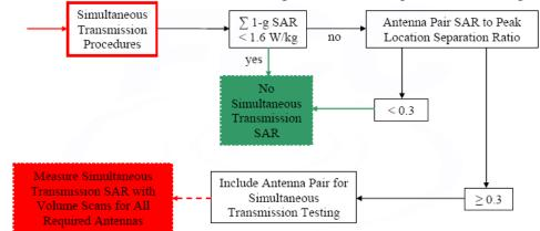
Fig. 3.1 KDB 648474 Simultaneous Transmission SAR Procedures for a Cell Phone
