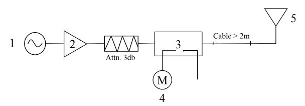
Fig. 8.1 System Setup for System Evaluation
