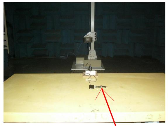
This part belongs to the interface(Jig+RS-232) of the control DUT.
