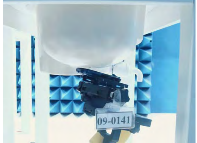
Figure 3. Right Head SAR Test Setup (Tilted)
