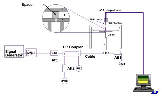
Fig. 8.1 System Setup for System Evaluation
