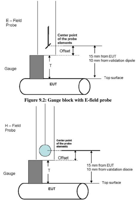
Figure 9.3: Gauge block with H-field probe
