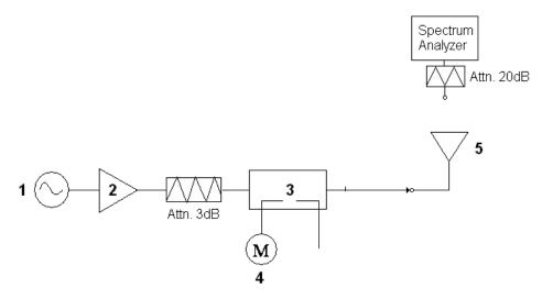
Fig. 8.1 System Calibration
