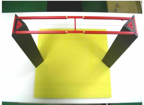
Fig. 5.7 Test Arch Phantom
