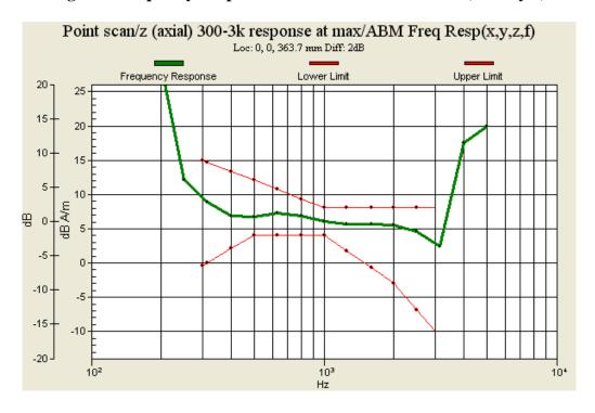
Fig. 9.8: Frequency Response of CDMA2000 PCS Ch600 (Battery 1)
