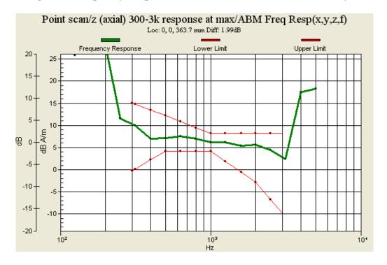
Fig. 9.12: Frequency Response of CDMA2000 PCS Ch1175 (Battery 2 and BT On)
