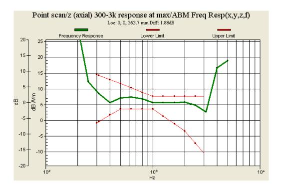
Fig. 9.5: Frequency Response of CDMA2000 Cellular Ch777 (Battery 3)
