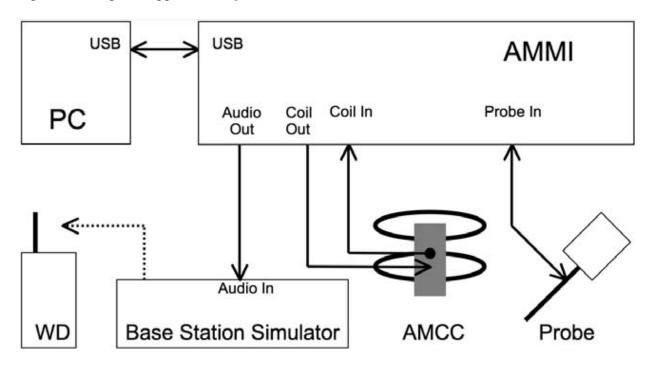
Fig. 5.7: T-Coil setup cabling
