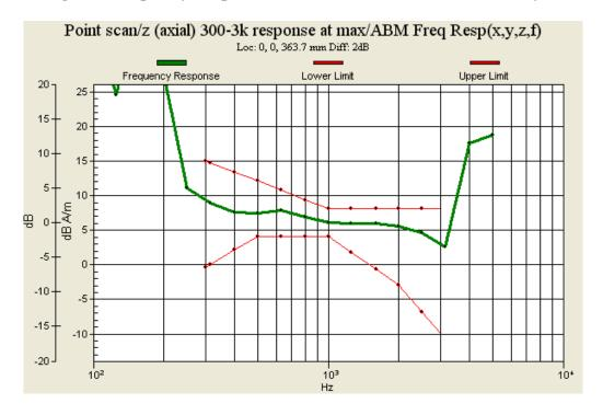
Fig. 9.10: Frequency Response of CDMA2000 PCS Ch1175 (Battery 2)
