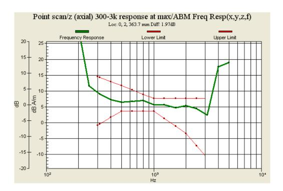
Fig. 9.7: Frequency Response of CDMA2000 PCS Ch25 (Battery 1)
