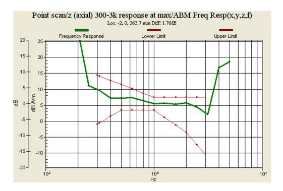
Fig. 9.3: Frequency Response of CDMA2000 Cellular Ch777 (Battery 1)
