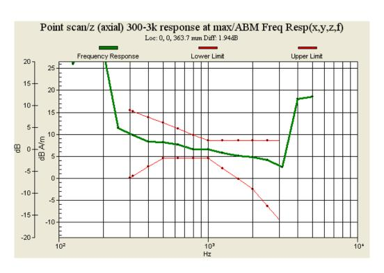
Fig. 9.9: Frequency Response of CDMA2000 PCS Ch1175 (Battery 1)
