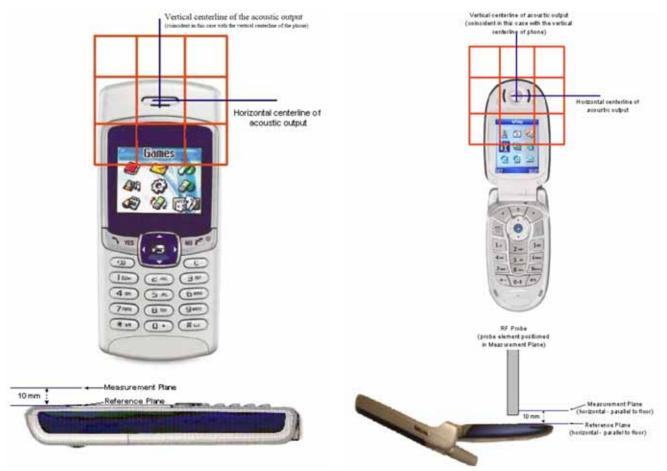
Fig. 6.1: A typical DUT reference and plane for HAC measurements
