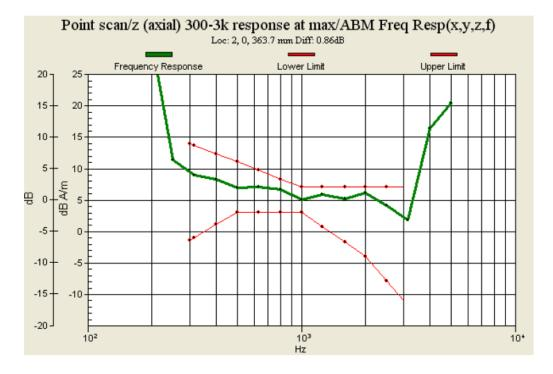
Fig. 9.6: Frequency Response of CDMA2000 Cellular Ch777 (Battery 1 and BT On)
