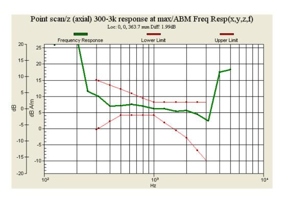
Fig. 9.11: Frequency Response of CDMA2000 PCS Ch1175 (Battery 3)
