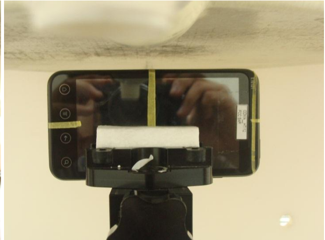
Left Side of the DUT with Phantom 0.5 cm Gap for DUT without Earphone
