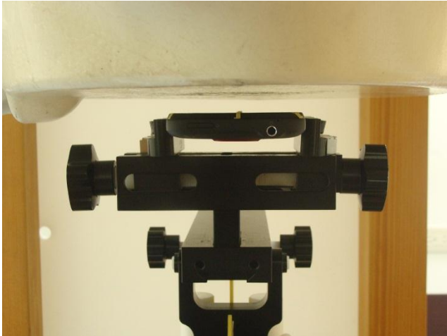
Front Face of the DUT with Phantom 1.0 cm Gap for DUT without Earphone
