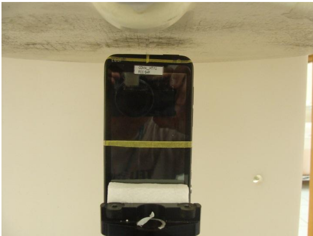
Top Side of the DUT with Phantom 1.0 cm Gap for DUT without Earphone
