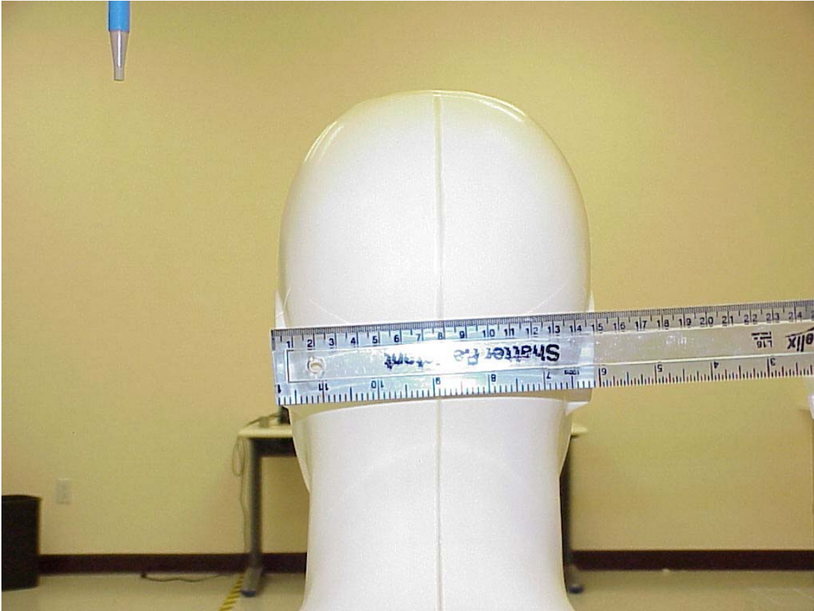
Photo 8. Photo to demonstrate 15 cm Z-axis head phantom
