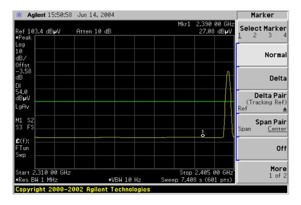
Detector mode: Peak Polarity: Horizontal
