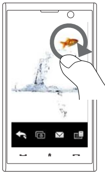
Slide your finger clockwise on an area to zoom in on that area.
