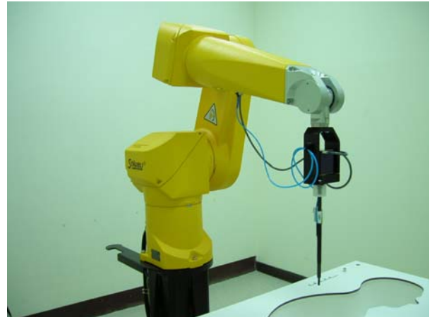
Fig. 5.2 Probe setup on robot
